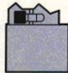
Lo-boy furnace unit on return air.
