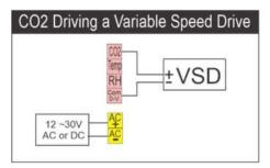
In this example a standard Variable Speed Drive is being controlled with the CO2 0-10V output. The Installer menu permits you to scale the 0-10V output to match your requirements such as output 0V at 450ppm and output 10V at 800ppm.
