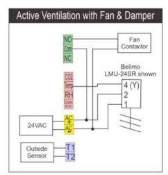
If you would like, you can have both the temperature 0-10V output and volt free relay used for advanced ventilation. In the Active Ventilation Output options menu settings select both relay and temp 0-10 (option 3). This permits you to open the fresh air damper and turn a fan on for example if outside air is suitable.
