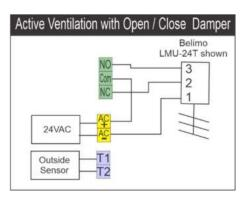
If selected in the Active Ventilation options menu, the monitor will modulate the temperature 0-10V output so that the output is at the maximum voltage set when the room temperature is 1 degree above the inside temperature setpoint. If introducing outside air the icon "A" will flash on the LCD. Tapping the "A" icon will briefly show the outside air temperature.
