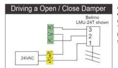
An open/close or an off/on output can be controlled by the monitor using the volt free relay provided. The relay threshold can be individually adjusted for each sensor. (30V @ 1A max)
