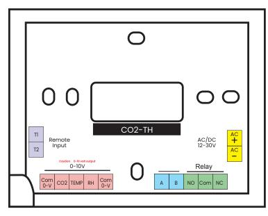
AC/DC The CO2-TH is powered from 12 to 30V AC or DC. If powering with DC +ve is applied to the top terminal and -ve is applied to the bottom
