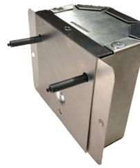
Use the external adapter plate when installing the Orion system to metal duct work. First rotate the probes 90 degrees. Use the supplied self tapping 10-32-1/4" screw. Attaching the plate ensures that there will be no air leakage from the duct work after the installation.
