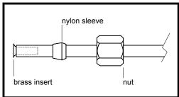
Finally, install a brass insert into the end of the plastic tubing.
