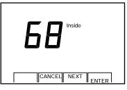
Press the Enter key to save the calibration and return to normal thermostat operation.
