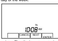
Press the Enter key when complete. The display returns to the normal time and temperature display.
